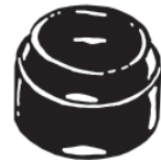
Center Post Upper Seal O.D. - 1 9/16" I.D. - 1 3/16" Thickness - 9/16"
